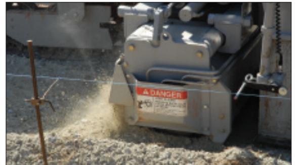
Trimmer gearbox and end plate are removable as a unit, making servicing easier
