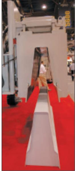
Molds can be mounted on the right side of the new 5700-C. This barrier mold is shown with the hydraulic barrier mold lift option.
