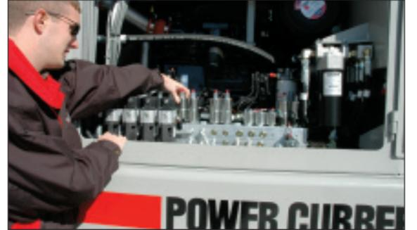
Servo valves are within easy reach. Pumps and gear box are more accessible for servicing
