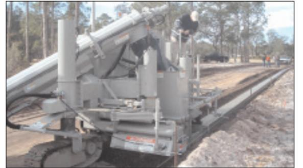
The re-positioned trimmer results in quicker set-up. The trimmer can be mounted 7 inches (18cm) further to the left, allowing the ability to trim and pour 6-foot (1.8m) sidewalk
