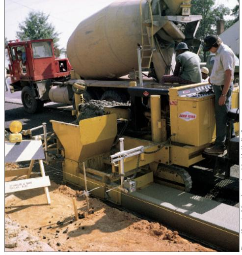
The Curb King 6500, the first slipform paver manufactured by Power Curbers, Inc., was the first machine to pour in the offset position, now an industry standard. The Curb King was the second curb machine that Ken used.
