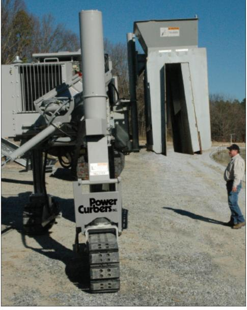
New option allows barrier mold to be elevated 5 feet (12.7cm) in the air
