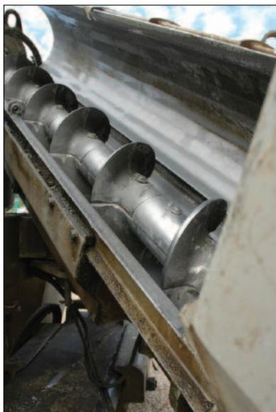
Machine clean-up is always important and can save you time and money. This auger flighting is on a well-cared-for machine that has more than 4,000 hours on it. The machine is owned by Pantano Concrete of York, PA
