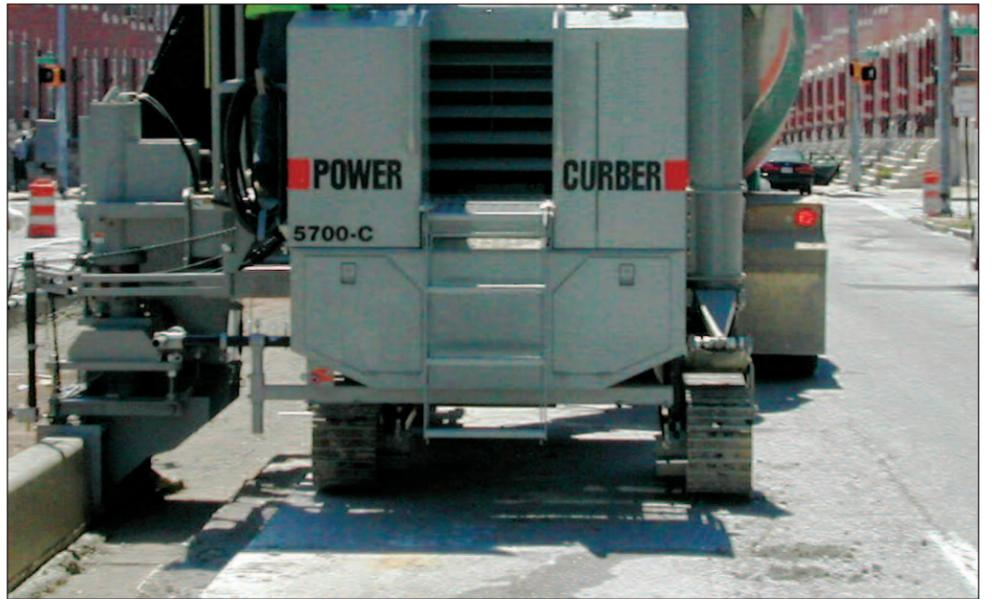
The repositioned auger on the 5700-C allows for single-lane pouring. This has come in very handy for Domti Engineering while slipforming curb in urban areas. The operator can line up the concrete truck directly in front of the machine for single-lane pouring in smaller, high-traffic volume areas such as city streets.
