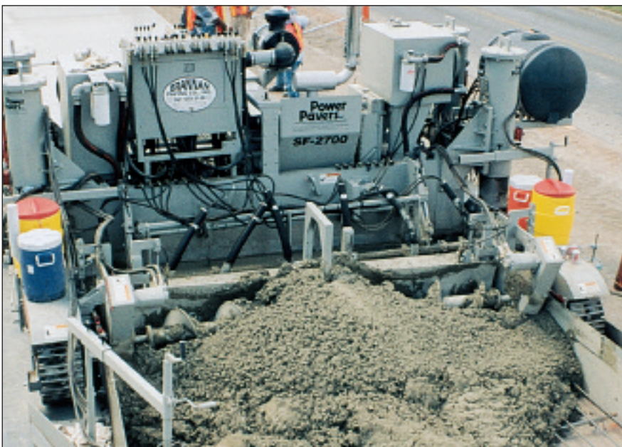
The SF 2700 features a dual controlled split auger system for spreading the mix evenly into the vibration chamber
