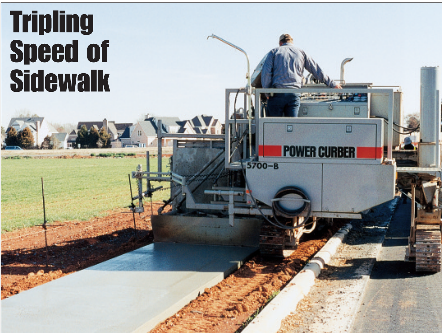
Nixon Curb & Gutter of Belmont, NC, has the new twin tank 5700-B. The rear-mounted twin tanks increase water capacity to 86 gal (322 l) and fuel capacity to 48 gal (185 l). In addition to the increased capacity, the setup makes it easier to re-fill the fuel tank
