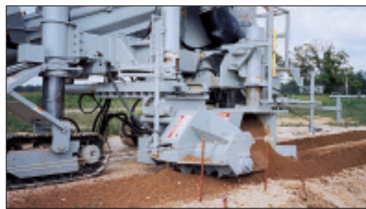
The trimmer digs a trench 10 inches deep (25 cm) and 6 inches wide (15 cm) and has the ability to trim an additional 12 inches (30 cm) on each side for clean-up
