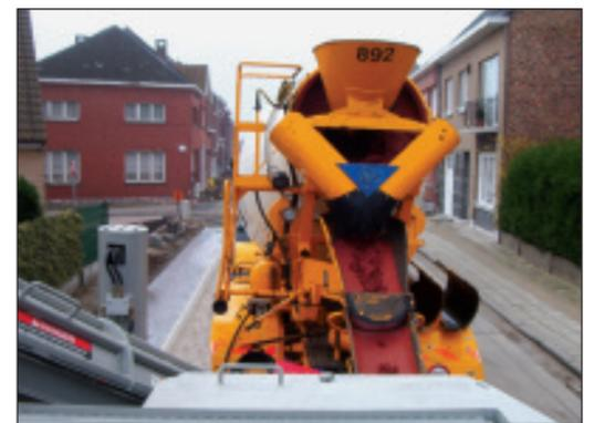
Power Curbers' new optional Swivel Auger allows the machine operator to angle the auger so that it is within easy reach of the truck. The concrete then drops directly into the hopper from this new angle.
