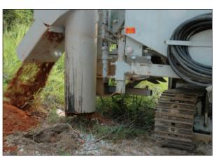
Material in hinged chute is displaced and does not fall back into the
