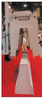
Molds can be mounted on the right side of the new 5700-C. This barrier mold is shown with the hydraulic barrier mold lift option.
