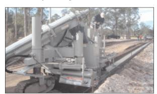
The re-positioned trimmer results in quicker set-up. The trimmer can be mounted 7 inches (18cm) further to the left, allowing the ability to trim and pour 6-foot (1.8m) sidewalk
