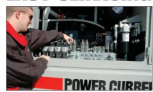
Servo valves are within easy reach. Pumps and gear box are more accessible for servicing
