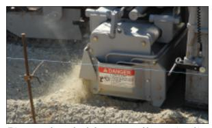
Trimmer gearbox and end plate are removable as a unit, making servicing easier
