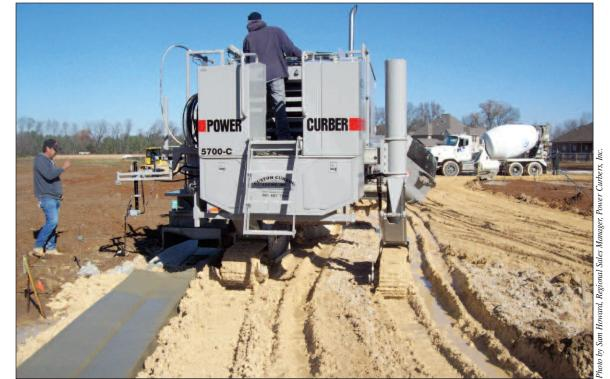
SUCCESS STORY: Power Curbers worked with Custom Curb & Edging, widening the tracks on the front and left crawlers to 16 inches (40.6cm) to keep the machine from bogging down in soft soil and delaying production
