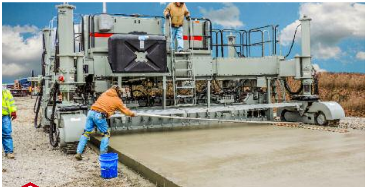
The wraparound walkway on the SF-2404 offers complete visibility of the machine's operation. Three ladders and a rear walkway provide easy access to the machine for operation and maintenance.
