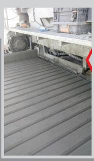
The paving kit on the Power Paver SF-2700 is able to include the floor and integrated curbs on both sides all in one pass, saving time and money
