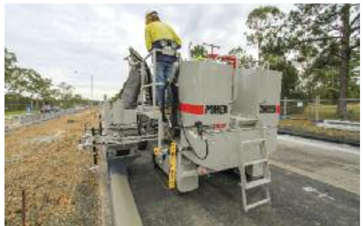
The rear post on the 5700-C-MAX can be returned to its standard position for pouring curb and gutter. Optional crawler guards shown.
