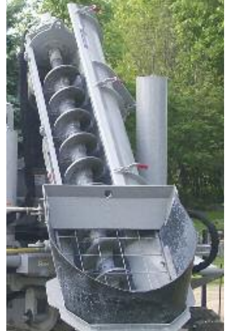
Auger Conveyor; lid opens for cleaning.
