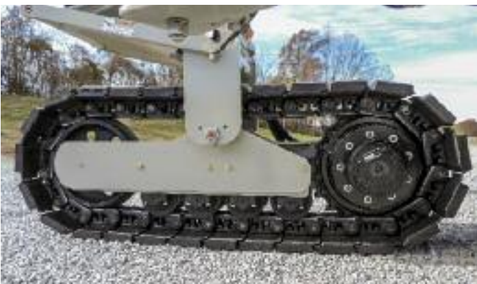
Close-up of MAX Package crawlers with polyurethane pads.
