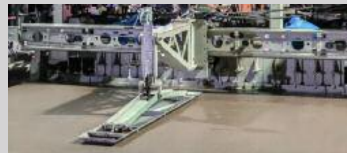
Optional Final Finisher. Oscillating mechanical float, adjustable to match the paving width.
