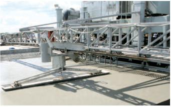
Optional final finisher features an oscillation mechanical float.
