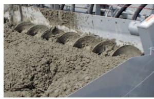
The spread auger and strike-off plate.
