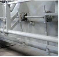
Tamper bar and vibrator mount/lift.
