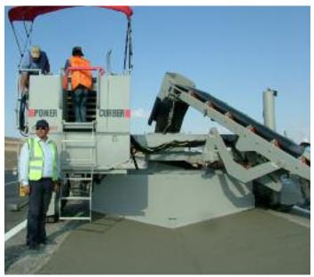
Ditch Liner in Turkey, 12.5' (3.8m) wide and 2' (.6m) deep, adjacent to pavement on both sides. (shown with custom belt conveyor)
