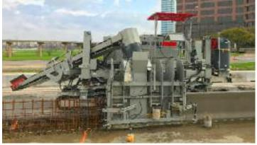
A Power Curbers 7700 Multipurpose Slipform Machine Pouring Variable Barrier
