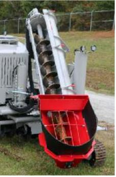
Auger Conveyor; lid opens for cleaning.
