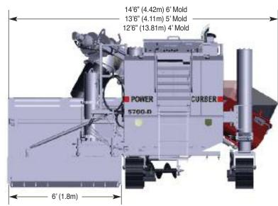
Machine with a 6' (1.8m) wide Sidewalk Mold.
