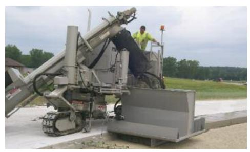
Apron addition over steel, sensing off existing pavement.
