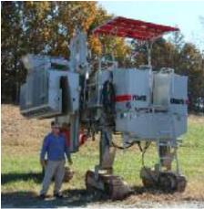
5700-D-MAX equipped with barrier mold lift.
